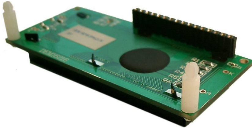
Figure 18: Spacers of the display
