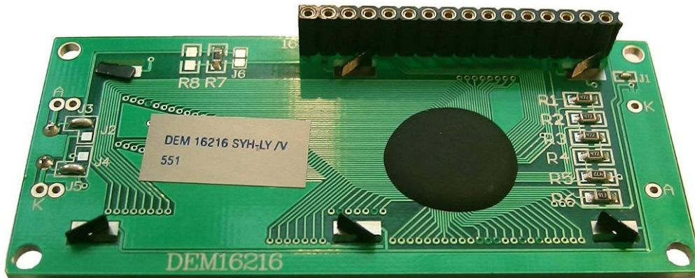
Figure 16: The 16 pole female connector strip at the lower edge of the display
